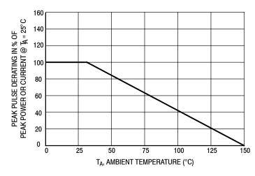
Figure 3. Pulse Derating Curve
