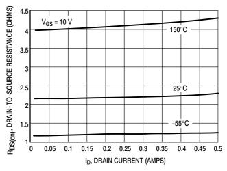
Figure 8. On-Resistance versus Drain Current
