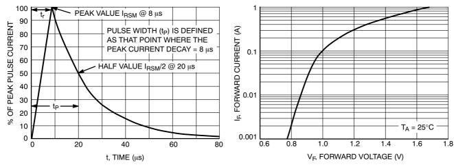
Figure 3.  $8\times 20~\mu s$  Pulse Waveform
