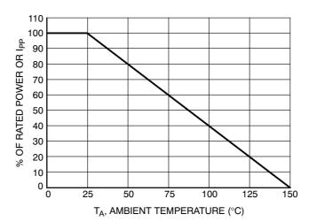
Figure 5. Power Derating Curve
