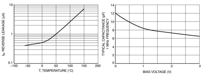
Figure 1. Reverse Leakage versus Temperature
