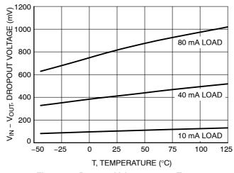
Figure 10. Dropout Voltage versus Temperature
