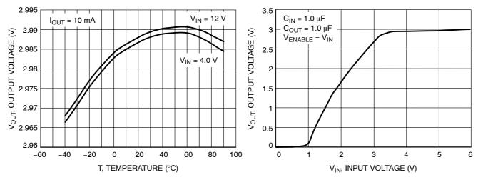
Figure 8. Output Voltage versus Temperature
