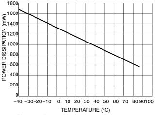
Figure 2. Power Dissipation vs Temperature
