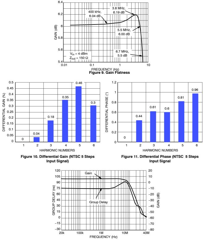
Figure 12. Normalized Frequency Response and Group Delay vs. Frequency
