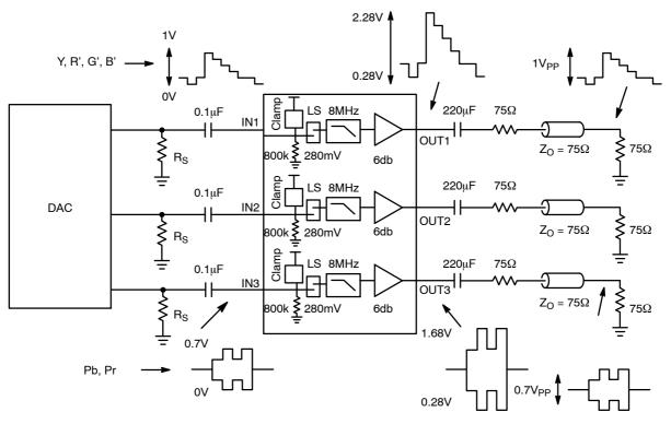
Figure 13. AC-Coupled Inputs and Outputs
