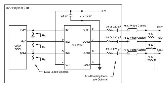
Figure 14. Typical Application Circuit
