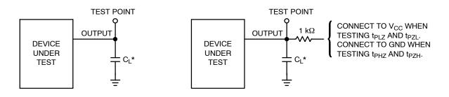
\*Includes all probe and jig capacitance
