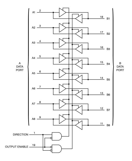
Figure 7. Expanded Logic Diagram
