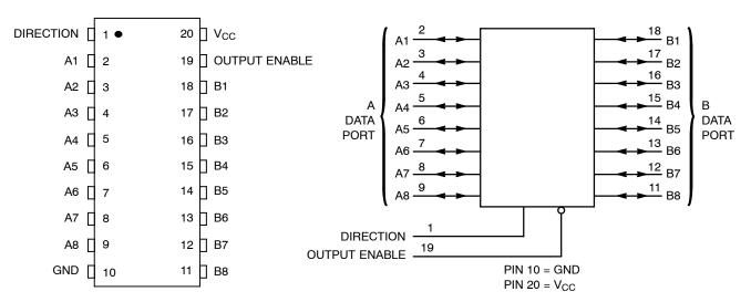
Figure 1. Pin Assignment
