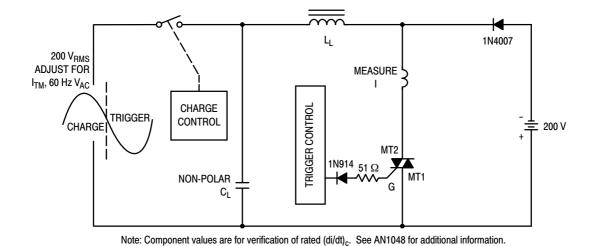
Figure 9. Simplified Test Circuit to Measure the Critical Rate of Rise of Commutating Current (di/dt)<sub>c</sub>
