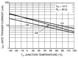
**Figure 6. Gate Trigger Current Variation**
