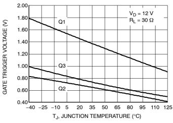
Figure 7. Gate Trigger Voltage Variation
