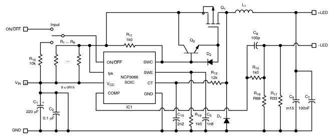
Figure 15. Buck Demoboard with External Switch Application Schematic
