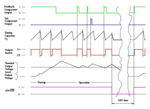
Figure 12. Typical Operating Waveforms
