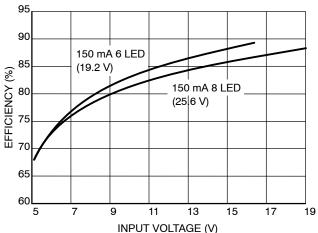
Figure 25. Boost LED Driver Efficiency
