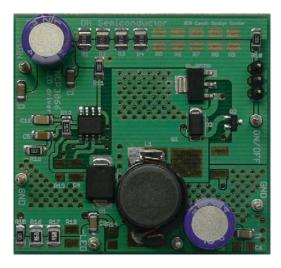
Figure 17. Buck with External Switch Demoboard Photo
