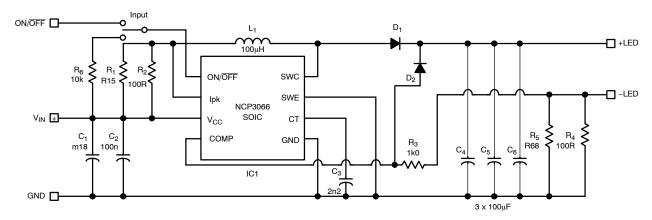
Figure 22. Boost demoboard Application Schematic
