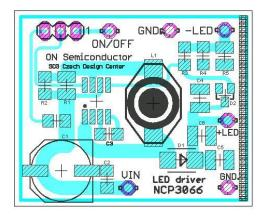
Figure 23. Boost Demoboard Layout
