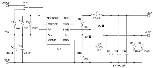
Figure 27. Buck Demoboard Application Schematic
