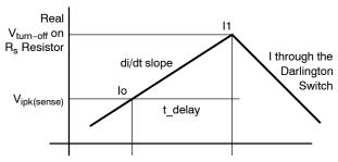
Figure 13. Current Sense Waveform
