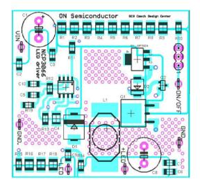
Figure 16. Buck with External Switch Demoboard Layout
