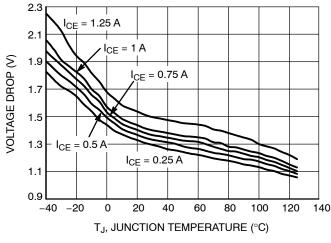
Figure 7. Voltage Drop in Emitter Follower Configuration
