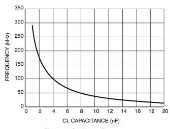
Figure 5. Oscillator Frequency vs.
