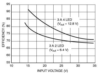
Figure 19. Efficiency of Buck LED Driver at I<sub>out</sub> = 3 A
