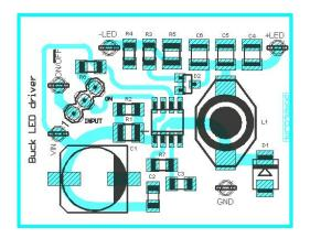
Figure 28. Buck Demoboard Layout
