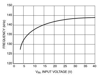
Figure 6. Oscillator Frequency vs. Supply Voltage
