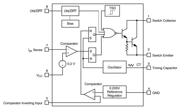
Figure 4. Block Diagram
