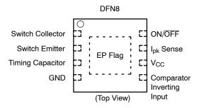
NOTE: EP Flag must be tied to GND Pin 4 on PCB
