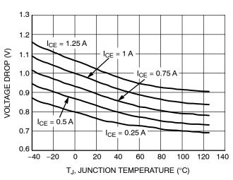
Figure 8. Common Emitter Configuration Output Darlington Switch Voltage Drop vs. Temperature
