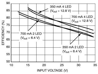
Figure 18. Efficiency of Buck LED Driver
