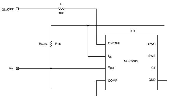
Figure 32. ONOFF Serial Resistor Connection
