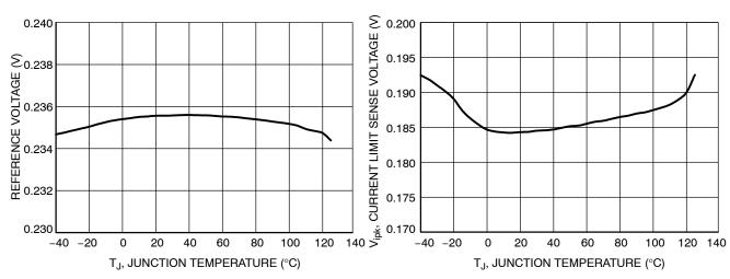
Figure 9.  $V_{th}$  vs. Temperature
