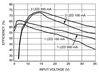
Figure 31. Efficiency of Buck LED Driver
