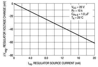
Figure 10. Regulator Output Voltage Change versus Source Current
