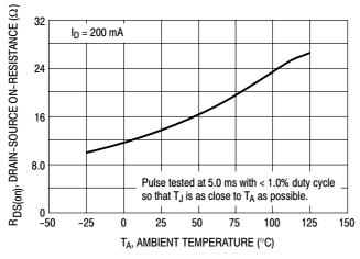
Figure 12. Power Switch Drain-Source On-Resistance versus Temperature
