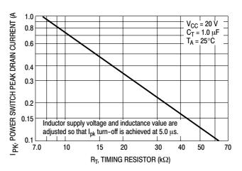
Figure 3. Power Switch Peak Drain Current versus Timing Resistor
