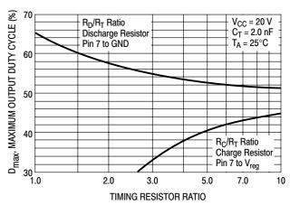
Figure 5. Maximum Output Duty Cycle versus Timing Resistor Ratio
