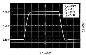
Figure 9. Error Amplifier Large Signal Transient Response
