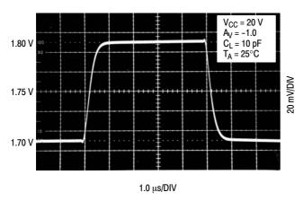
Figure 8. Error Amplifier Small Signal Transient Response
