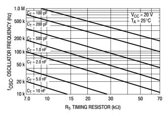
Figure 2. Oscillator Frequency versus Timing Resistor
