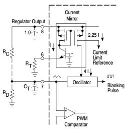
Figure 21. Maximum Duty Cycle Modification
