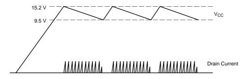
Figure 20. Timing Diagram of Short-Circuit Condition
