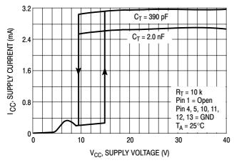
Figure 14. Supply Current versus Supply Voltage
