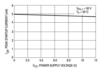
Figure 11. Peak Startup Current versus Power Supply Voltage
