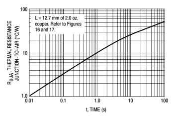
Figure 15. DW and P Suffix Transient Thermal Resistance
