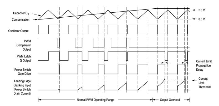
Figure 18. Timing Diagram of Normal Operation
