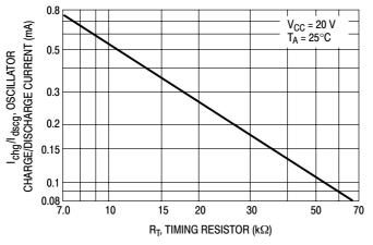
Figure 4. Oscillator Charge/Discharge Current versus Timing Resistor
