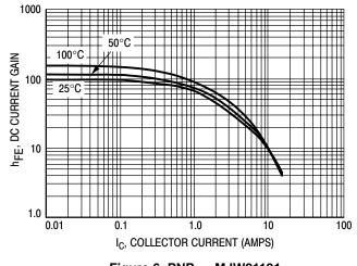
Figure 6. PNP — MJW21191 V<sub>CE</sub> = 2.0 V DC Current Gain
