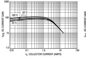
Figure 5. NPN — MJW21192 V<sub>CE</sub> = 2.0 V DC Current Gain PNP — MJW21191
