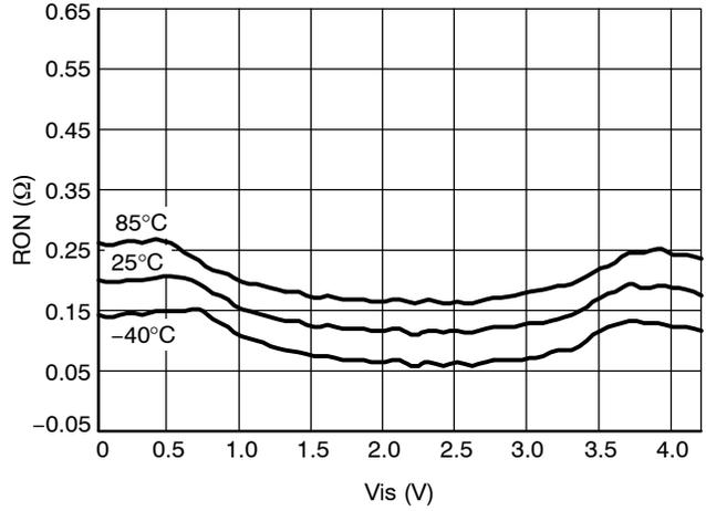
Figure 2. RON vs. Vin @ Vcc = 4.3 V, All Temps
