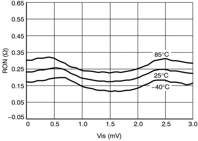
Figure 1. RON vs. Vin @ Vcc = 3.0 V, All Temps
