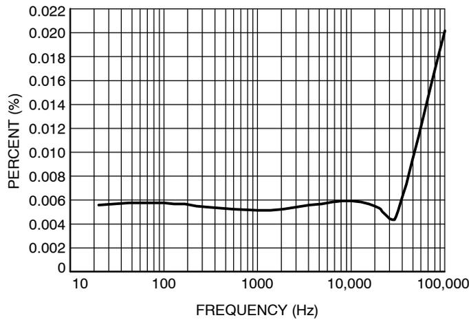
Figure 5. THD vs. Frequency @ Vin = 1 Vpp
