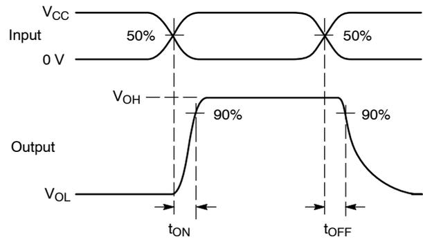
Figure 7.  $t_{ON}/t_{OFF}$
