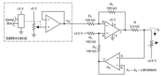
Figure 13. Programmable Current Source/Sink
