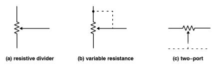
Figure 5. Potentiometer Configuration
