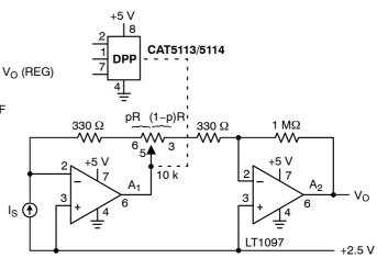
Figure 10. Programmable I to V Converter
