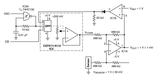
Figure 8. Sensor Auto Referencing Circuit
