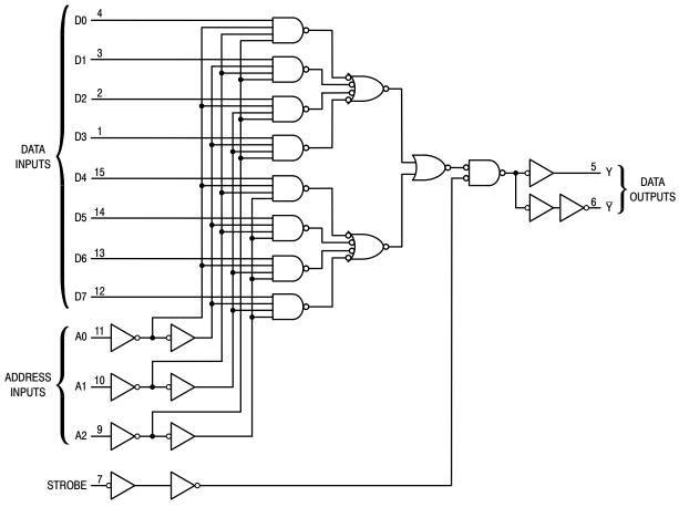
Figure 8. Expanded Logic Diagram
