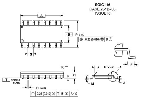
NOTES: 1. DIMENSIONING AND TOLERANCING PER ANSI Y14.5M, 1982. 2. CONTROLLING DIMENSION: MILLIMETER. 3. DIMENSIONS A AND B DO NOT INCLUDE MOLD PROTRUSION. 4. MAXIMUM MOLD PROTRUSION 0.15 (0.006) PER SIDE. 5. DIMENSION D DOES NOT INCLUDE DAMBAR PROTRUSION. ALLOWABLE DAMBAR PROTRUSION SHAIT RE 0.127 (0.005) TOTAL IN EXCESS OF THE D SHALL BE 0.127 (0.005) TOTAL IN EXCESS OF THE D DIMENSION AT MAXIMUM MATERIAL CONDITION.
