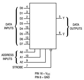
Figure 1. Logic Diagram
