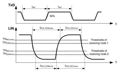
Figure 6. LIN Transmitter Duty Cycle
