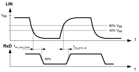
Figure 9. LIN Receiver Timing
