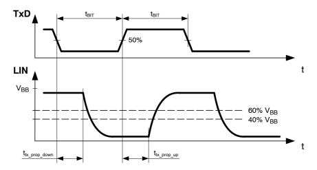
Figure 7. LIN Transmitter Timing
