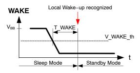
Figure 4. Local Wake-up Detection
