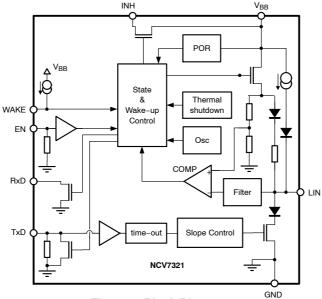
Figure 1. Block Diagram
