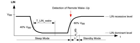
Figure 5. Remote (LIN) Wake-up Detection
