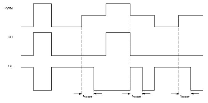
Figure 5. Tri-State Operation
