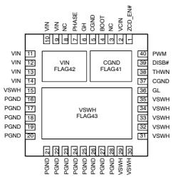
Figure 3. Pin Connections (Top View)
