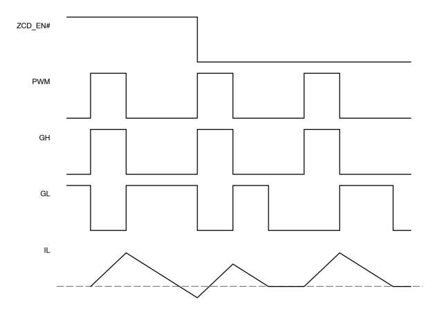
Figure 4. Zero Current Detection
