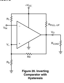
When  $V_{IN}$  is less than the voltage at the non-inverting node,  $V_+$ , the output voltage will be high. When  $V_{IN}$  is greater than the voltage at  $V_+$ , then the output will be low. The hysteresis band (Figure 21) created from the resistor network is defined as:
