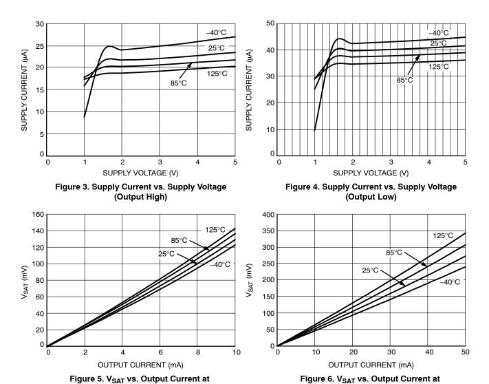
$V_{CC} = 5.0 \text{ V}$
