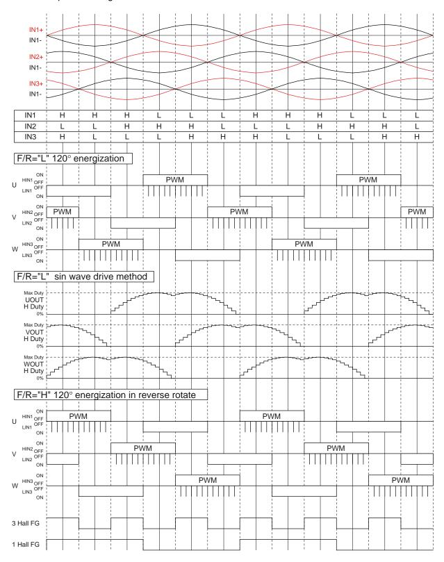
The energization is switched to 120° wher 3 Hall FG frequency is 5.15Hz (typ) or lower A direction of rotation is detected from Hall signal according to F/R pin input If the motor rotates in reverse against F/R pin input 120° energization is maintained forcibly
