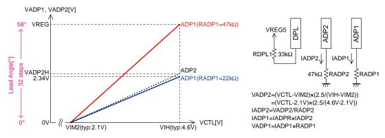
2. The ADP2 pin rise can be halted (a limit on the lead angle adjustment can be set by means of the CTL voltage) by setting DPL (pin 10).
