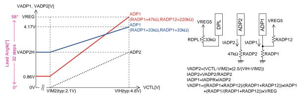
4. When the lead angle is not adjusted
