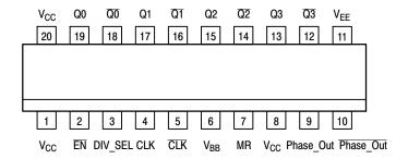
Figure 1. Pinout: 20-Lead SOIC (Top View)
