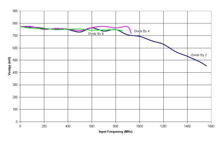
Figure 4. Fmax: Voutpp vs Input Frequency per DIV2/4/6
