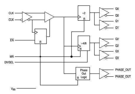
Figure 2. Logic Diagram
