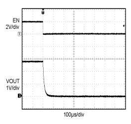
Figure 17. Enable Turn-off (500 mA Load)
