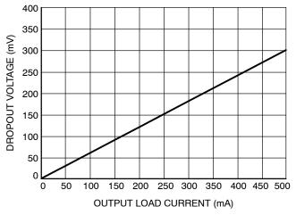
Figure 11. Dropout vs. Load Current
