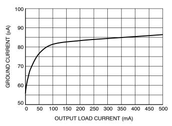
Figure 9. Ground Current vs. Load Current
