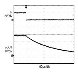
Figure 15. Enable Turn-off (100 μA Load)
