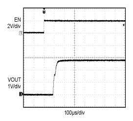
Figure 16. Enable Turn-on (500 mA Load)
