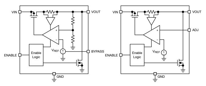
Figure 20. Block Diagram – Fixed Voltage
