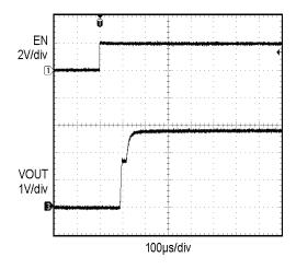
Figure 14. Enable Turn-on (100 μA Load)
