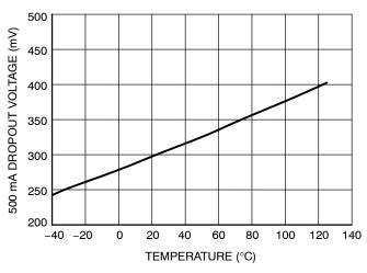
Figure 10. Dropout vs. Temperature (500 mA Load)
