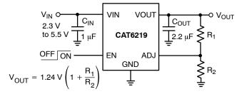
Figure 2. Adjustable Output LDO
