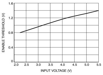
Figure 12. Enable Threshold vs. Input Voltage
