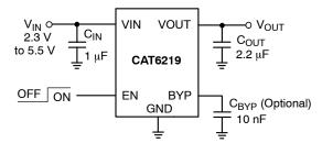
Figure 1. Typical Application Circuit
