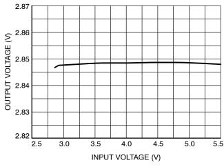
Figure 3. Dropout Characteristics
