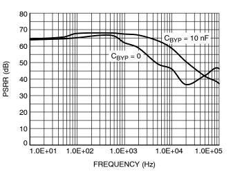
Figure 13. PSRR vs. Frequency (10 mA Load)
