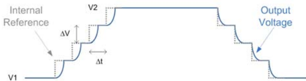
Figure 21. Dynamic Voltage Scaling Effect Timing Diagram
