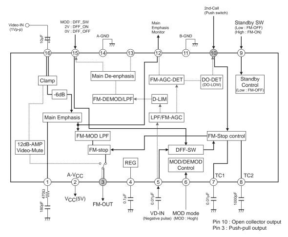
Application Circuit Example2 Demodulation (Monitor)
