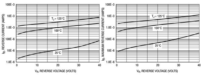
Figure 3. Typical Reverse Current
