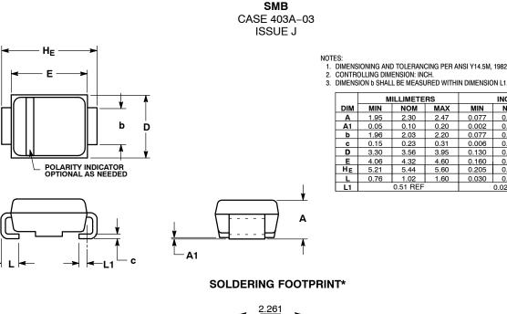
DIMENSIONING AND TOLERANCING PER ANSI Y14.5M, 1982.
