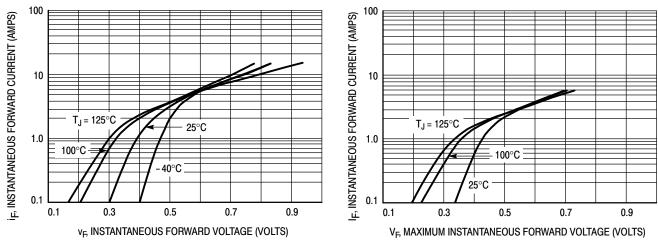
Figure 1. Typical Forward Voltage
