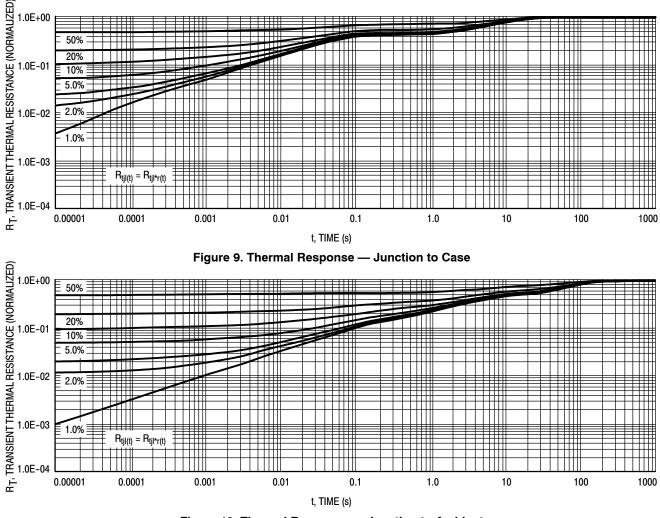
Figure 10. Thermal Response — Junction to Ambient
