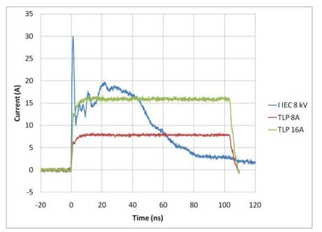
Figure 15. Comparison Between 8 kV IEC 61000-4-2 and 8 A and 16 A TLP Waveforms
