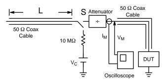
Figure 14. Simplified Schematic of a Typical TLP System
