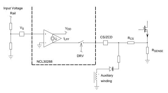
Figure 8. Line Feed–Forward Schematic
