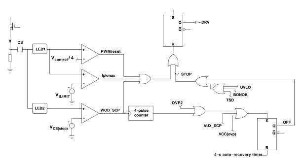
Figure 9. Winding Short Circuit Protection, Max. Peak Current Limit Circuits
