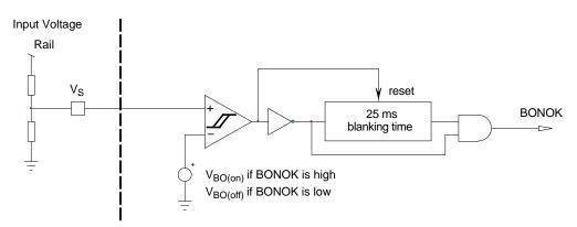
Figure 10. Brown-out Protection Circuit
