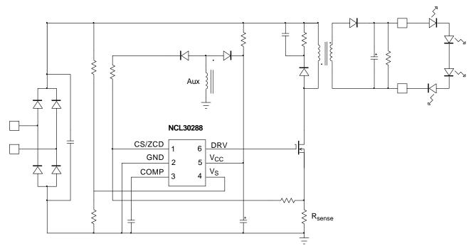
Figure 1. Typical Application Schematic in a Flyback Converter
