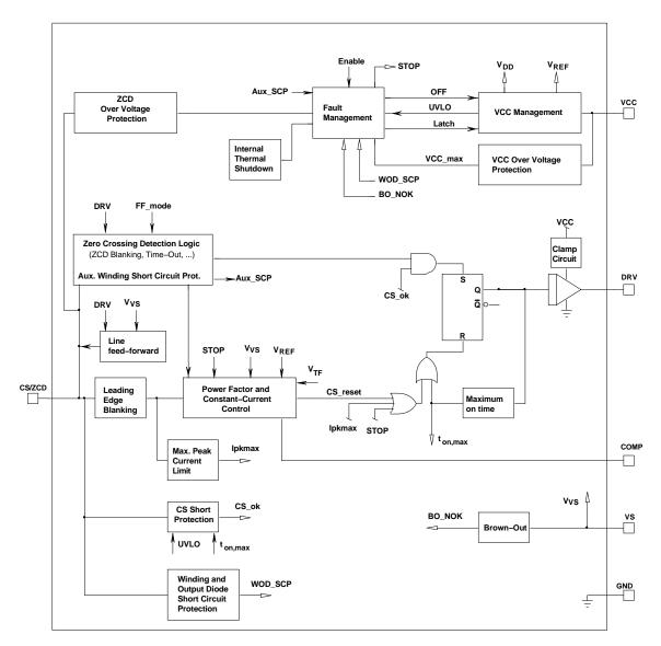
Figure 3. Internal Circuit Architecture
