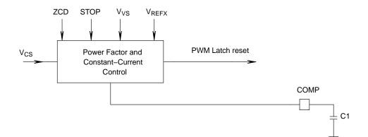
Figure 4. Power Factor and Constant–Current Control
