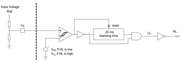
Figure 6. Line Range Detection Circuitry
