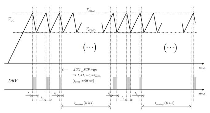
Figure 5. Start-up Sequence in a Load Short-circuit Situation
