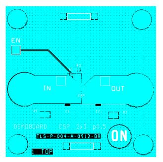
Figure 12. Demoboard PCB Top View
