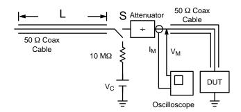
Figure 9. Simplified Schematic of a Typical TLP System
