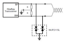
Figure 7. FlexRay Surge Protection Circuit
