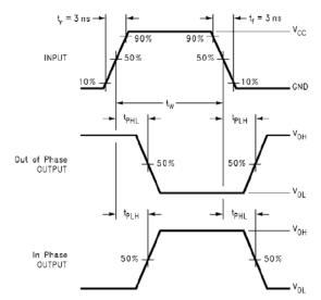
Figure 16. AC Waveforms
