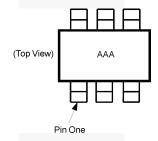
Figure 3. Pin 1 Orientation
