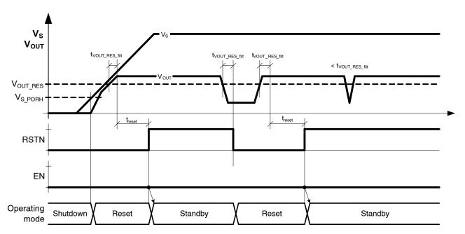
Figure 6. V<sub>OUT</sub> Regulator Voltage Monitoring
