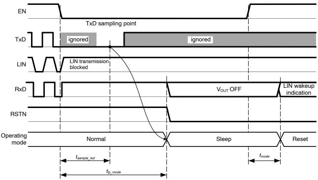
Figure 10. Operating Modes, Transition from Normal to Sleep Mode
