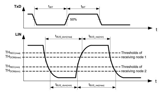
Figure 11. Definition of LIN Duty Cycle Parameters
