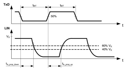
Figure 13. Definition of LIN Transmitter Timing Parameters
