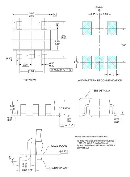
Figure 7. 5-Lead SOT23, JEDEC MO-178 1.6mm
