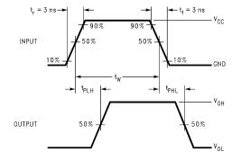
Figure 5. AC Waveforms
