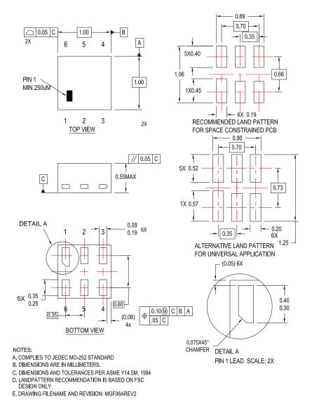
Figure 10. 6-Lead, MicroPak2, 1x1mm Body, .35mm Pitch
