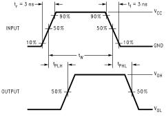
Figure 5. AC Waveforms
