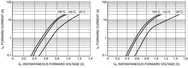
Figure 1. Typical Forward Voltage
