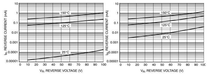
**Figure 3. Typical Reverse Current**
