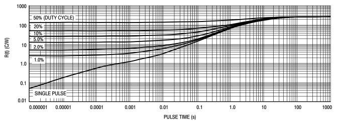
Figure 8. Thermal Response, Junction-to-Ambient (6 mm<sup>2</sup> pad)
