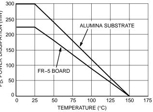
Figure 2. Steady State Power Derating Curve
