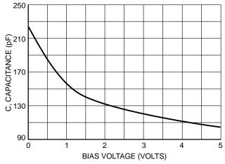
Figure 4. Typical Diode Capacitance (SM05)
