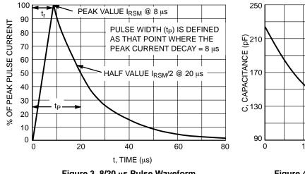
Figure 3. 8/20 µs Pulse Waveform
