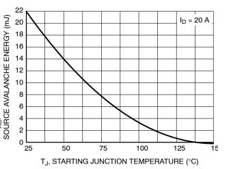
Figure 12. Maximum Avalanche Energy vs. Starting Junction Temperature
