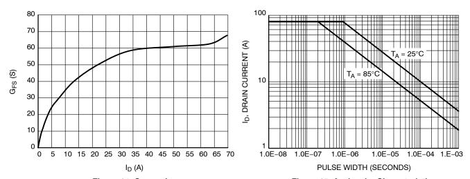
Figure 14.  $G_{FS}$  vs.  $I_D$
