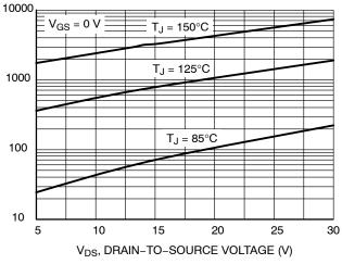
Figure 6. Drain-to-Source Leakage Current vs. Voltage
