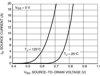
Figure 10. Diode Forward Voltage vs. Current
