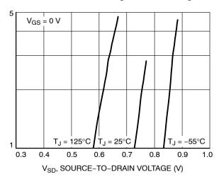
Figure 10. Diode Forward Voltage vs. Current
