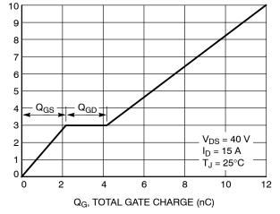
Figure 8. Gate-to-Source and Drain-to-Source Voltage vs. Total Charge
