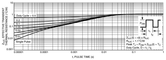
Figure 13. Junction-to-Case Transient Thermal Response Curve
