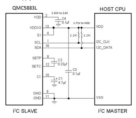
Figure 5. Dual Supply Connection
