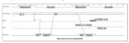
Figure 11 Data Read Sequence at Measurement
