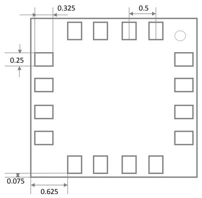
Figure 7. QMC5883L PCB footprint
