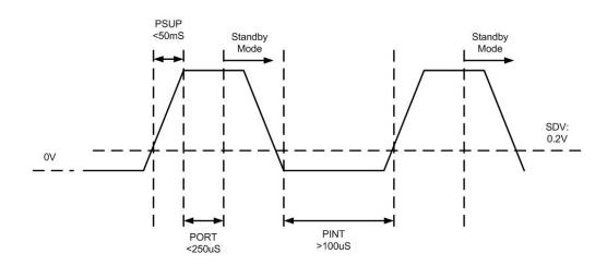
Figure 8. Power On/Off Timing
