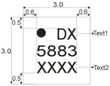
Figure 4. Chip Marking
