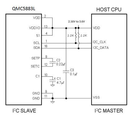
Figure 6. Single Supply Connection
