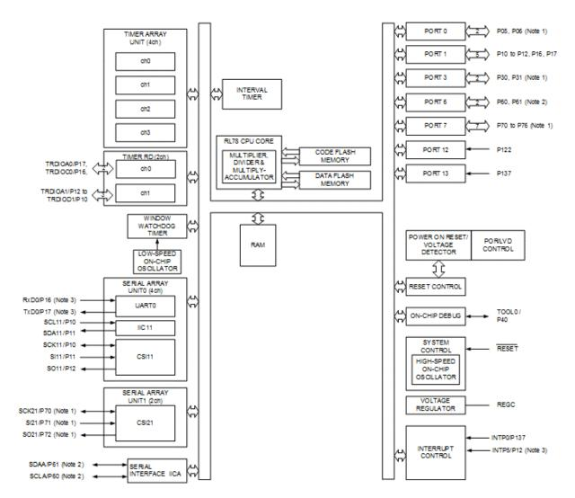
Note 1. P05, P06, P30, P31 and P70 to P76 are connected to AFE chip in the package. And are not connected to any external pins. Note 2. P60/SDAA0 is connected to SDA pin and P61/SCLA0 is connected to SCL pin respectively.
