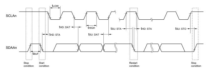
**IICA** serial transfer timing
