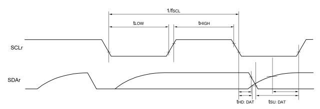
Simplified I<sup>2</sup>C mode serial transfer timing (during communication at same potential)
