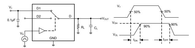
Test Circuit 2. Switching Times  $(t_{ON},\,t_{OFF})$
