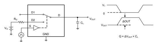
Test Circuit 4. Charge Injection
