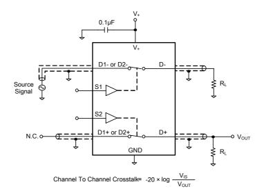
Test Circuit 6. Channel-to-Channel Crosstalk
