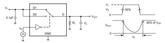
Test Circuit 3. Break-Before-Make Time Delay (t<sub>D</sub>)
