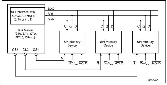
1. The Write Protect (W/V<sub>PP</sub>) and Hold (HOLD) signals should be driven, High or Low as appropriate.
