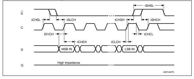
Figure 23. Serial Input Timing
