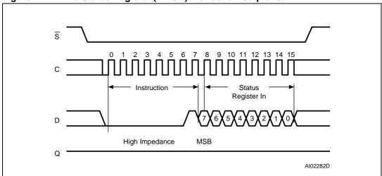
Figure 12. Write Status Register (WRSR) Instruction Sequence
