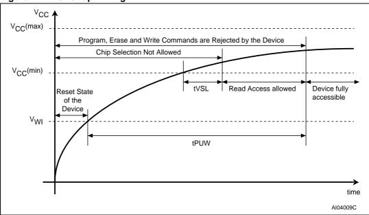
Figure 21. Power-up Timing
