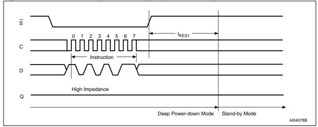
Figure 20. Release from Deep Power-down (RES) Instruction Sequence
