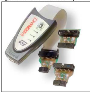
you to erase, program view and verify microcontroller memory. RFlasher also includes *automated mode* for automatic execution of programming sequences for mass programming and *project mode* that allows you to save your programming configuration.
