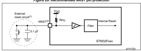
Figure 25. Recommended NRST pin protection
