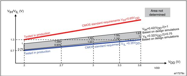
Figure 22. 5 V tolerant I/O input characteristics - CMOS port
