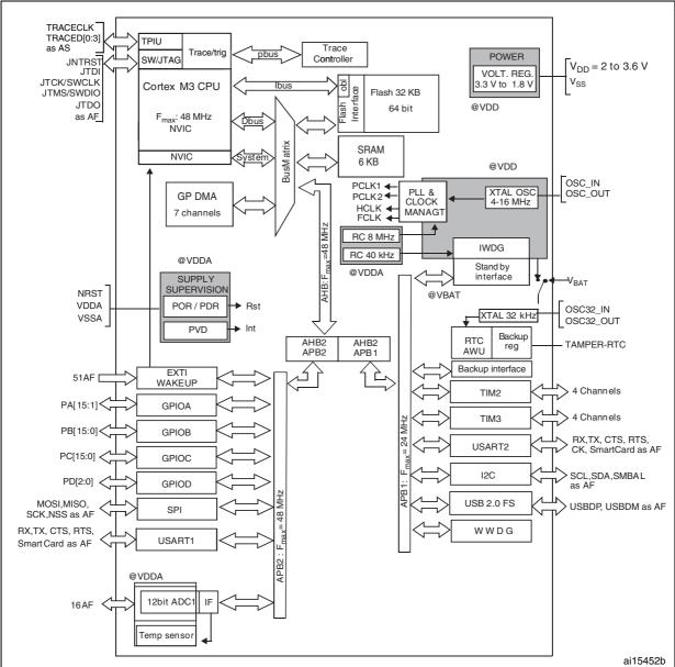
Figure 1. STM32F102T8 medium-density USB access line block diagram
