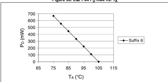
Figure 38. LQFP64 P<sub>D</sub> max vs. T<sub>A</sub>
