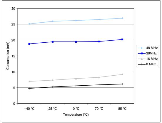
Figure 10. Typical current consumption in Run mode versus temperature (at 3.6 V) - code with data processing running from RAM, peripherals enabled
