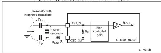
Figure 18. Typical application with an 8 MHz crystal
