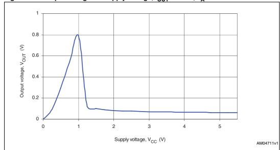
Figure 33. Output voltage vs. supply voltage,  $I_{OUT}$  = 1 mA,  $T_A$  = 25 °C
