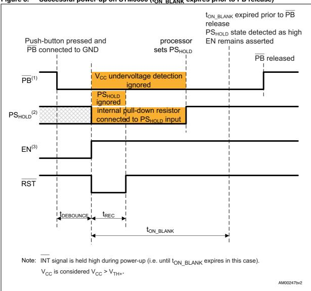
Figure 8. Successful power-up on STM6600 (t<sub>ON BLANK</sub> expires prior to PB release)
