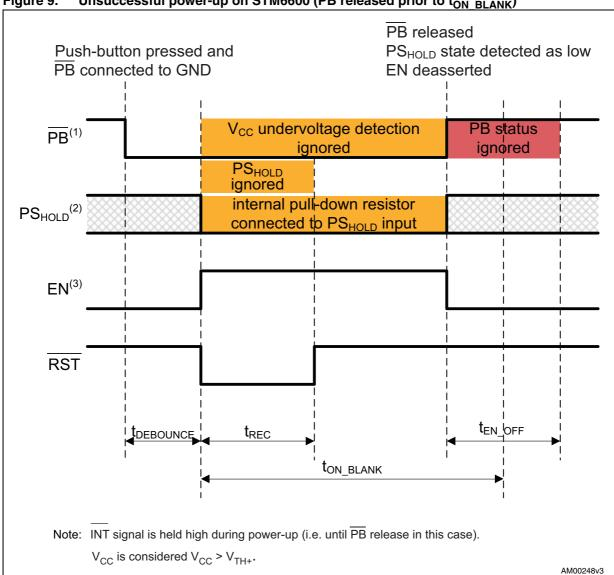
Unsuccessful power-up on STM6600 (PB released prior to ton BLANK) Figure 9.
