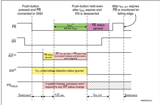
Figure 19. Long push (option with enable deassertion)
