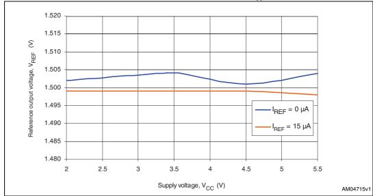
Figure 37. Reference output voltage vs. supply voltage,  $T_A = 25$  °C
