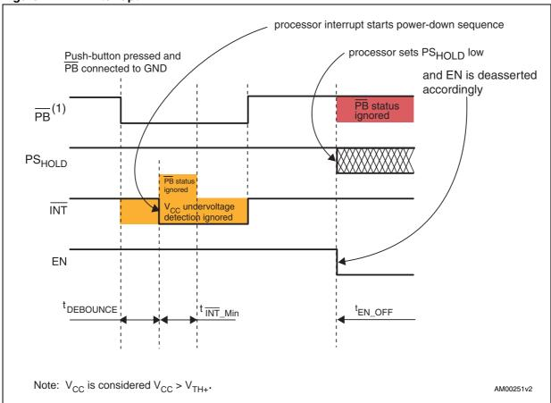
1. PB detection on falling edge.
