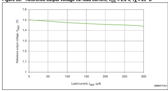
Figure 36. Reference output voltage vs. load current,  $V_{CC}$  = 2.0 V,  $T_A$  = 25 °C
