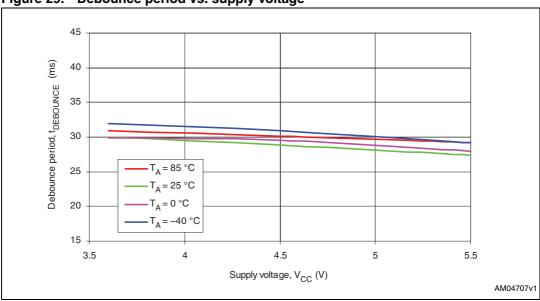
Figure 29. Debounce period vs. supply voltage
