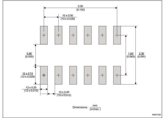
Figure 42. TDFN12 (2 x 3 mm) recommended footprint
