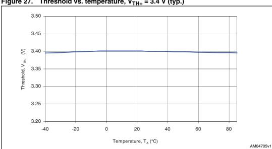
Figure 27. Threshold vs. temperature,  $V_{TH+} = 3.4 \text{ V (typ.)}$
