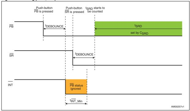
Figure 16. Long push, SR pressed first
