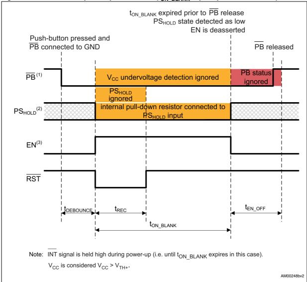
Figure 10. Unsuccessful power-up on STM6600 (ton Blank expires prior to PB release)
