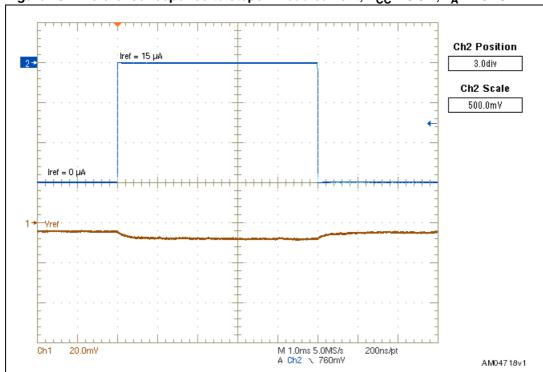
Figure 40. Reference response to steps in load current,  $V_{CC}$  = 3.6 V,  $T_A$  = 25 °C
