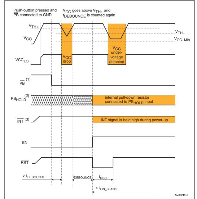
Figure 13. Power-up on STM660x with voltage dropout
