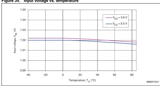
Figure 34. Input voltage vs. temperature
