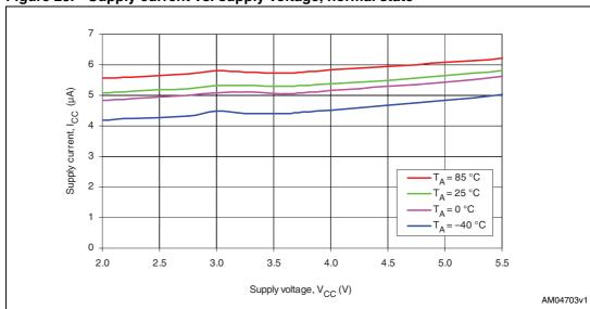
Figure 25. Supply current vs. supply voltage, normal state
