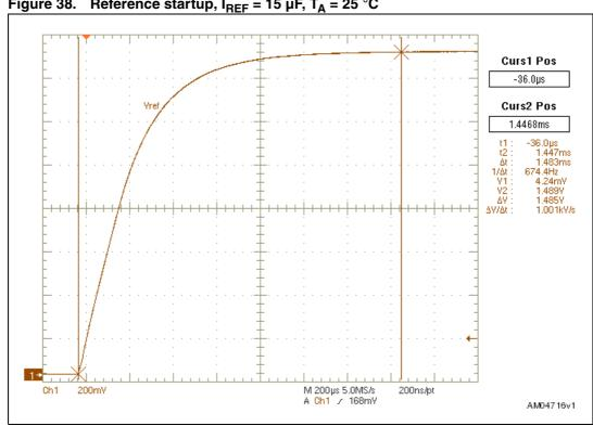
Figure 38. Reference startup,  $I_{REF}$  = 15  $\mu F$ ,  $T_A$  = 25  $^{\circ}C$
