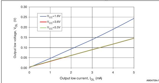
Figure 31. Output low voltage vs. output low current,  $T_A = 25^{\circ}C$
