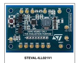
The generators can be externally programmed to sink up to 85 mA and can be dimmed via a PWM signal (1% of minimum dimming duty cycle at 1kHz can be managed).
