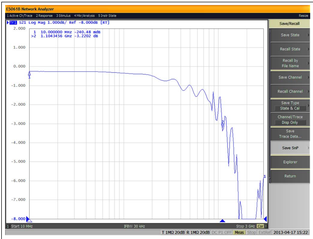
Figure 22. Data switch transfer characteristics vs. frequency
