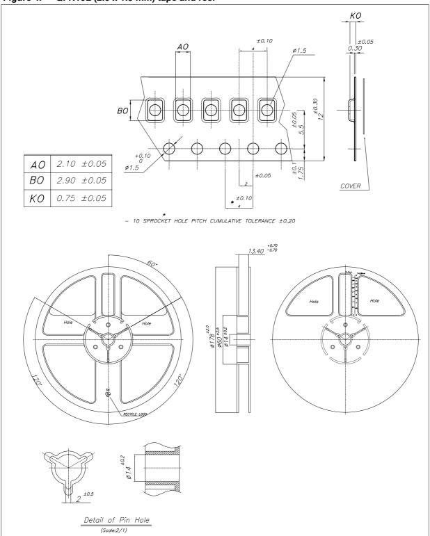
Figure 4. QFN16L (2.6 x 1.8 mm) tape and reel
