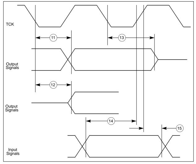
Figure 9. JTAG boundary scan timing
