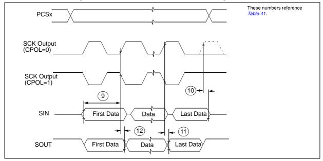
These numbers reference (3) Table 41. (2) SS SCK Input (CPOL=0) 4 4 SCK Input (CPOL=1) (12) (5 First Data Data Last Data SOUT (10) (9) First Data Data Last Data SIN
