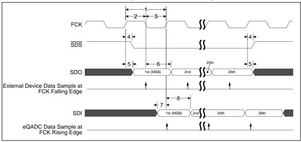
Figure 26. eQADC SSI timing
