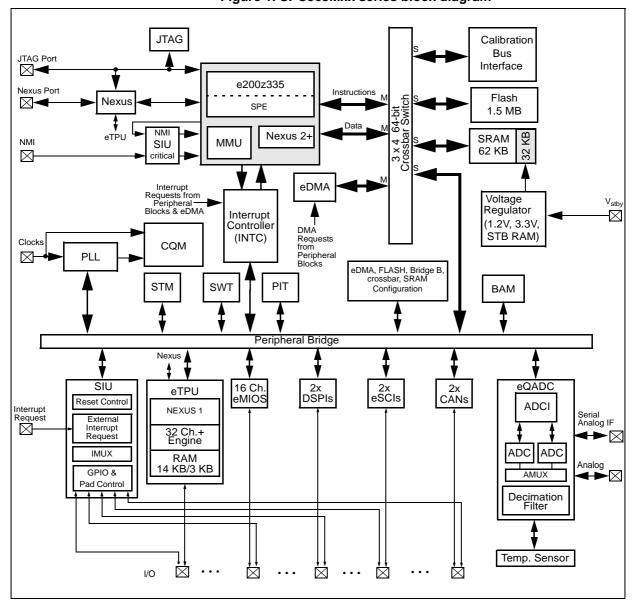
Figure 1. SPC563Mxx series block diagram
