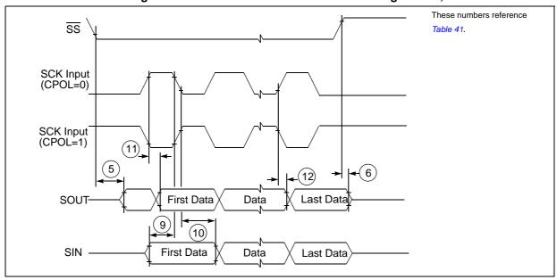
Figure 25. DSPI PCS strobe (PCSS) timing
