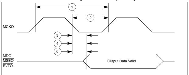
Figure 10. Nexus output timing
