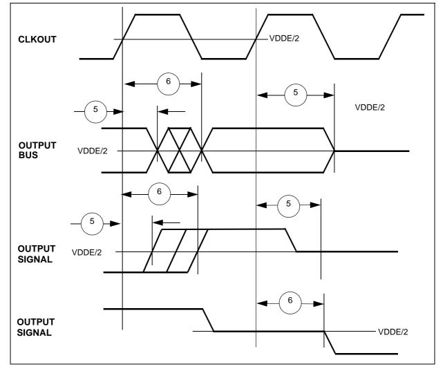
Figure 14. Synchronous output timing
