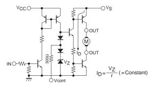
As shown in the left diagram, the Vcont pin outputs the voltage of the band gap Zener  $V_Z + V_F (= 1.93 \text{V})$ .
