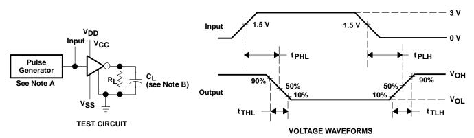
NOTES: A. The pulse generator has the following characteristics:  $t_W = 25 \mu s$ , PRR = 20 kHz,  $Z_O = 50 \Omega$ ,  $t_f = t_f < 50 ns$ .
