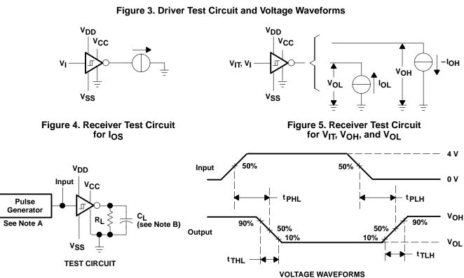
NOTES: A. The pulse generator has the following characteristics:  $t_W$  = 25  $\mu$ s, PRR = 20 kHz,  $Z_O$  = 50  $\Omega$ ,  $t_f$  =  $t_f$  < 50 ns.
