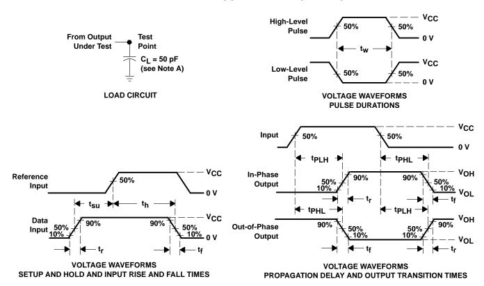
NOTES: A. C<sub>L</sub> includes probe and test-fixture capacitance.
